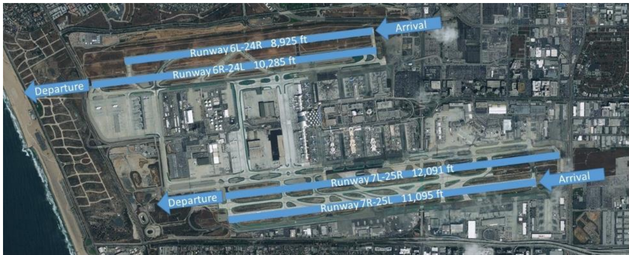
FIGURE 2-5: WEST FLOW OPERATIONS
