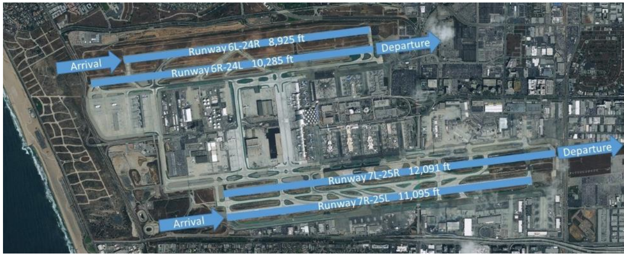
FIGURE 2-6: EAST FLOW OPERATIONS
