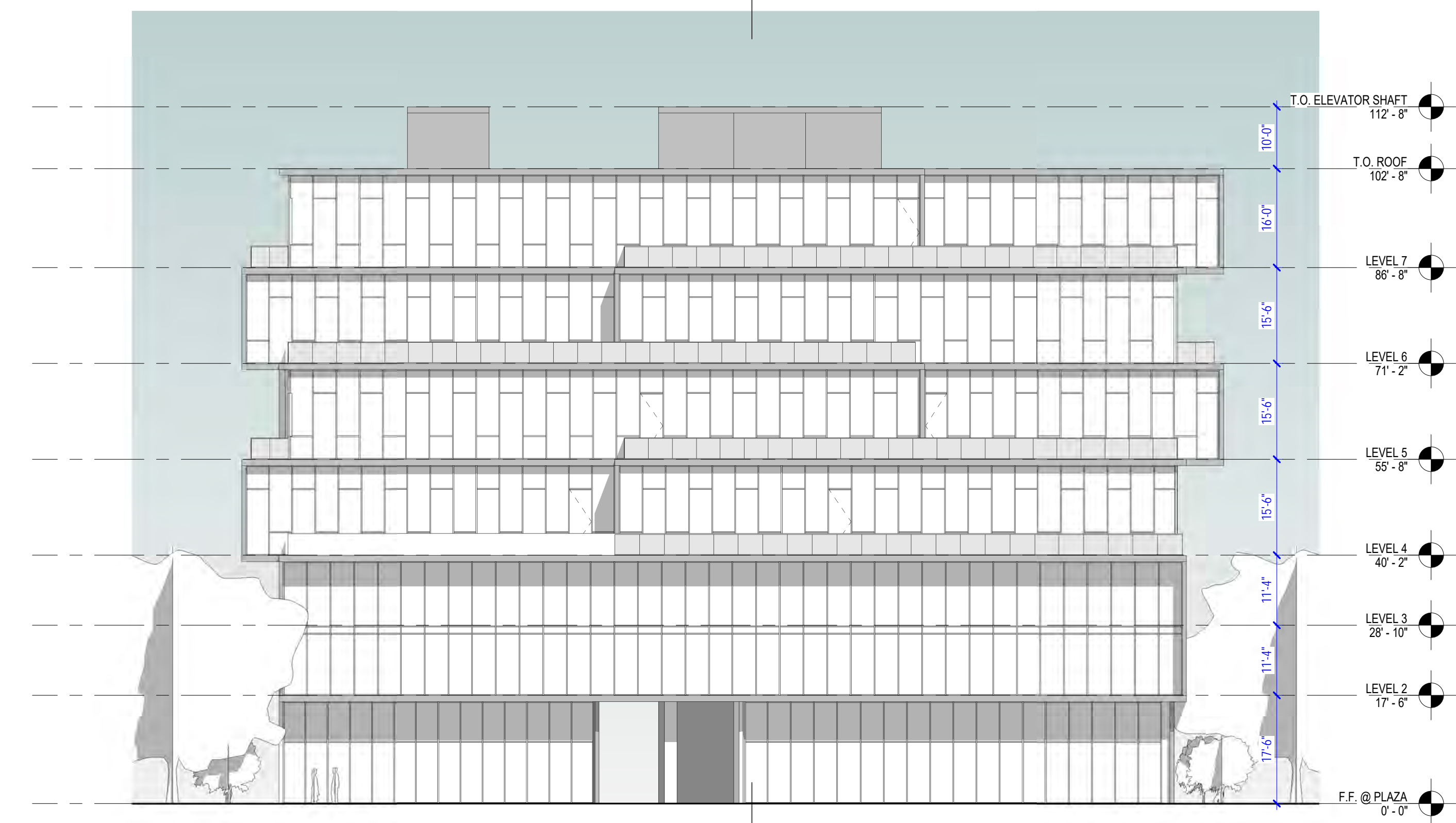
BUILDING C - WEST ELEVATION 01 SCALE: 1/16" = 1'-0"
